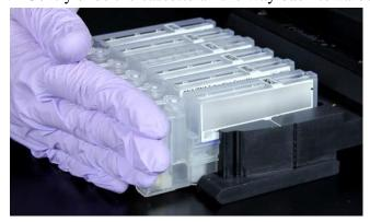
Do not use your index finger to push the cassette into the magazine. You may indirectly dispense the reagent. Luminex recommends using the palm of your hand to slide the cassette into proper position.
